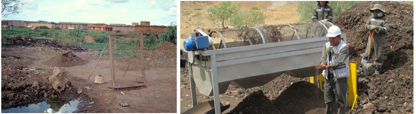
Figure 4. Sieve used at waste dump in Mali to produce compost and mechanized rotating sieve (source: WASTE and EAWAG)
